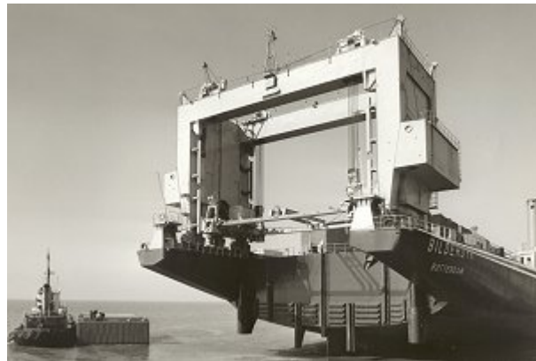
Stern embarkation of LASH barges by gantry crane
